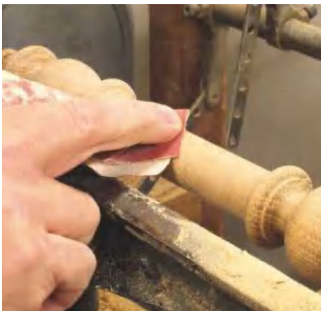
▲ Pic.25 Sand up the stem and when you have a parallel detail like I have here, it will be more efficient to stop the lathe and sand that area along the direction of the grain; this should stop those unsightly radial scratches that can appear
